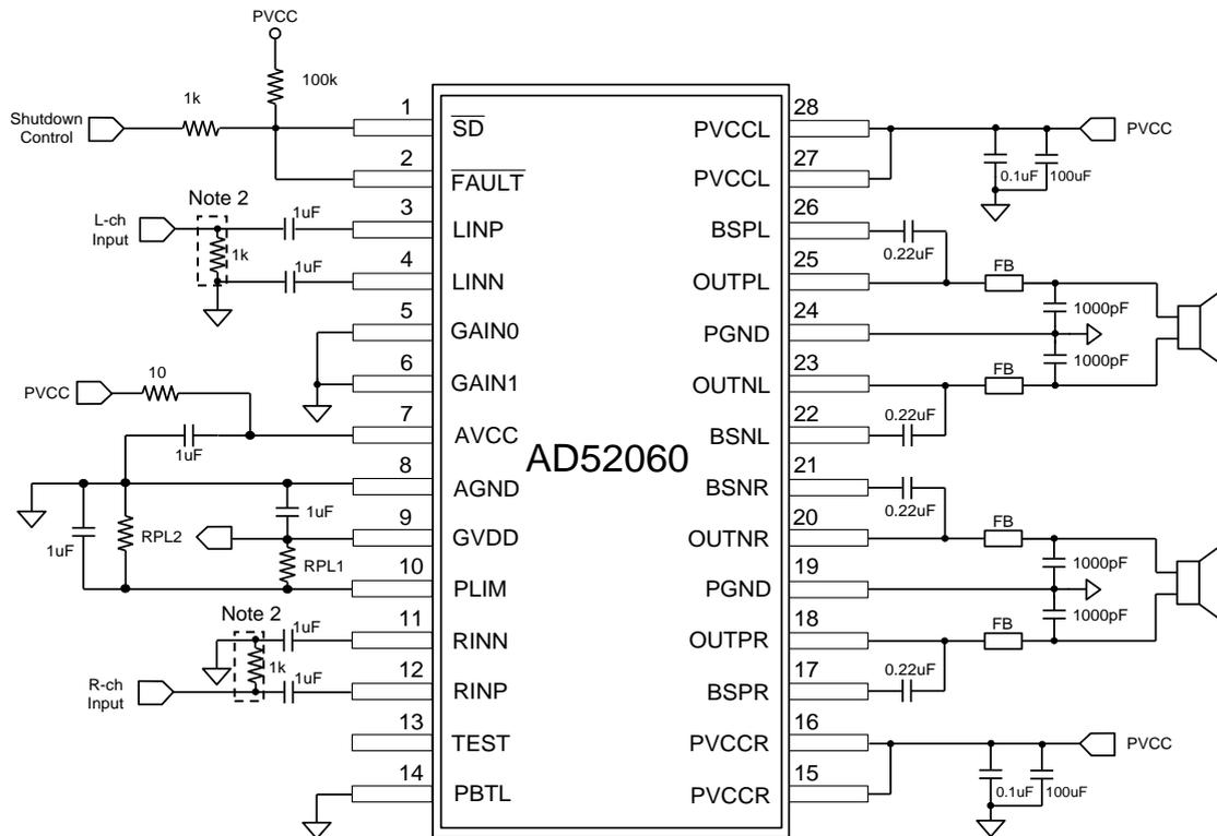
**Note 2:** These resistances must be connected to ground, resistance=1Kohm
