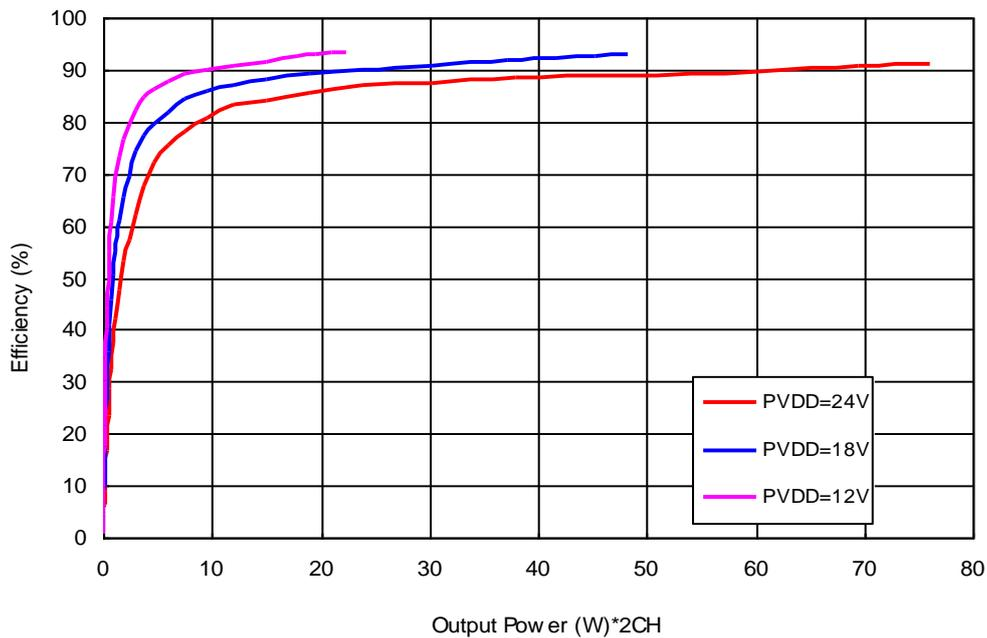
**Efficiency (Mono 4ohm load) / 2ch**
