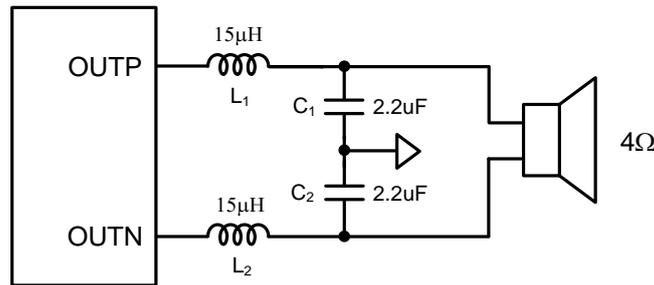
Figure 4. Typical LC Output Filter for 4Ω Speaker
