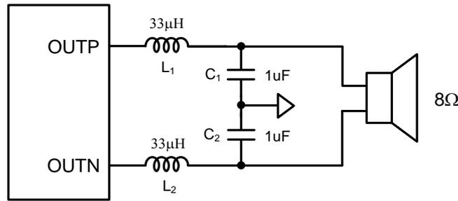
Figure 3. Typical LC Output Filter for 8Ω Speaker
